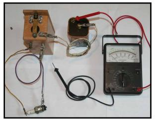
i. Adjusting the coil so that it draws between .85-.95 amps will make your coil and car happy. Lower amperages will give you a weak spark. Higher amperages will give you a huge spark, but will eventually burn out your coil.
